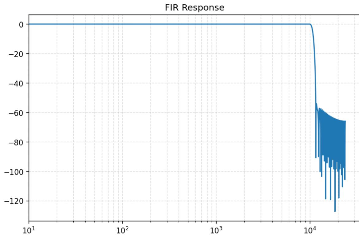
*The FIR stage removes high-frequency noise beyond the cutoff.*
