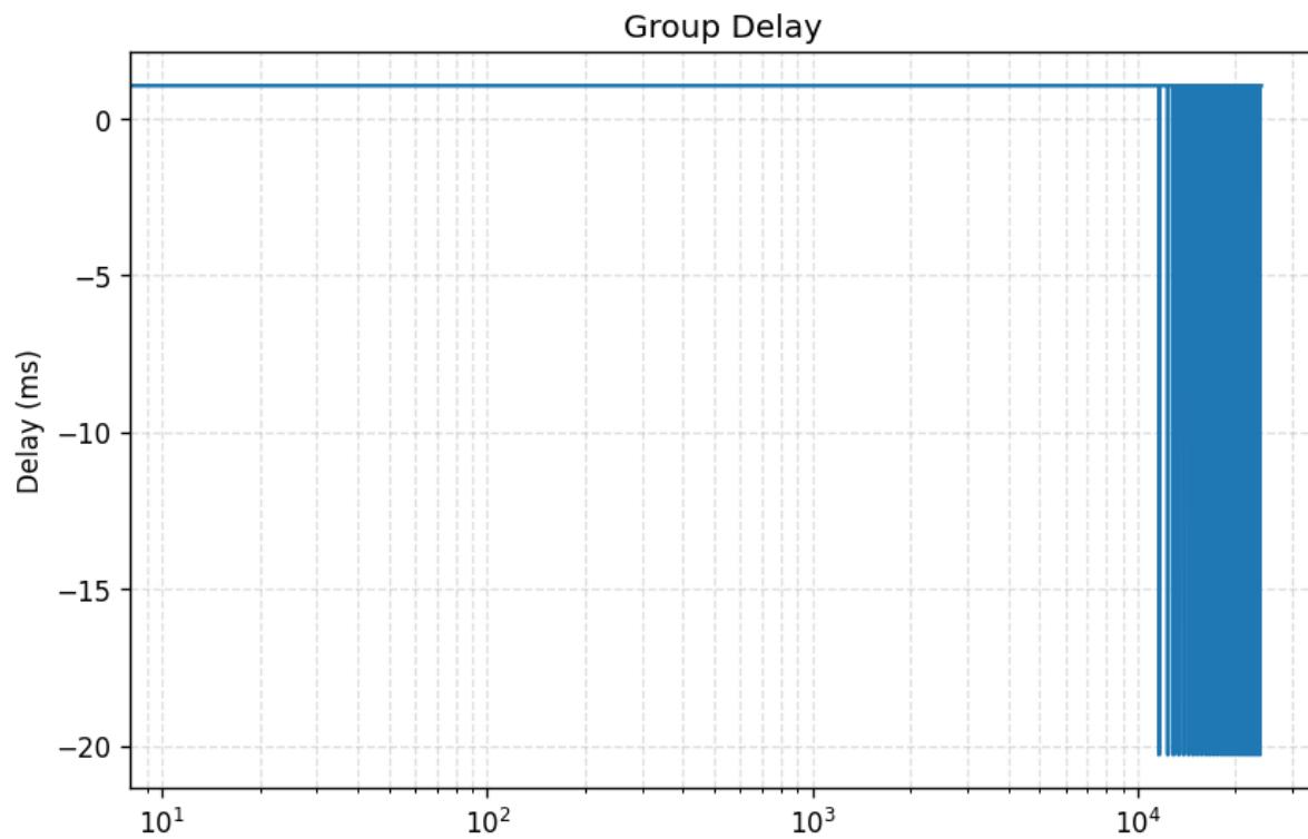
*Group delay spikes indicate the frequency of notch filters.*
