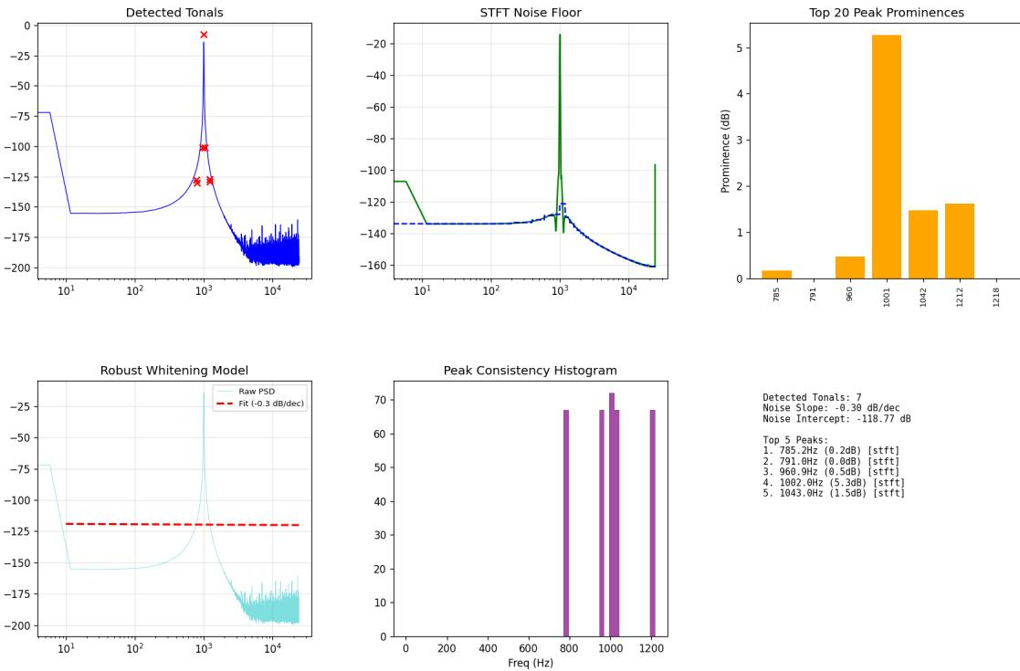
*Detailed breakdown of tonal detection showing thresholds, noise floors, and candidate evaluations.*
